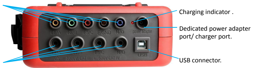
Figure 3-3: Connectors on the top of device
